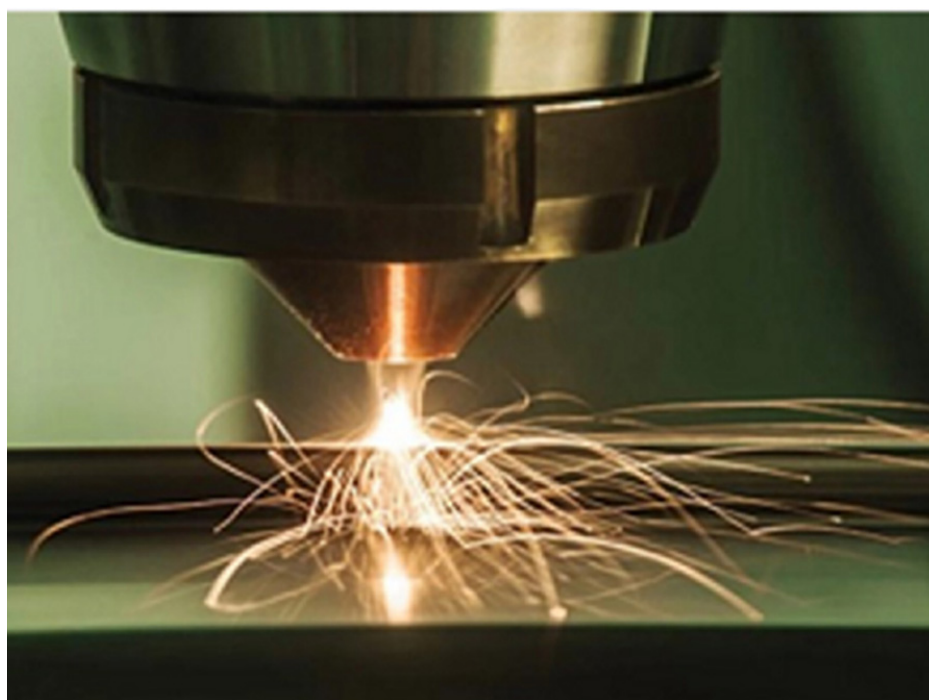
Figure 8. Illustration of a laser-powered DED process [46].
